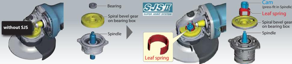
Absorption mechanism of vibration
