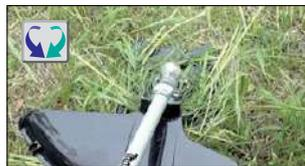
Reverse switch for easy removal of grass clippings from the cutting tool (UX01G / DUX60 only)
