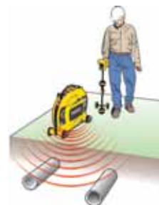
Induce a signal to locate utilities.
