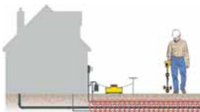
Direct connect to utility lines.
