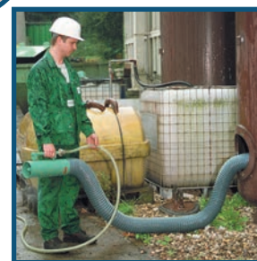
8 1620 0010 Pneumatic Air Mover, 7" dia. 2366 cfm output @ 90 psi
