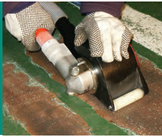
Air Models 194.0405 and 194.C405, 4" cutting width
