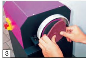
3 Uses the FIX HOOK AND LOOP SYSTEM (See pages 105-107). For replacement flap discs, see page 93.
