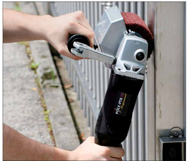
Satin finishing using interleaf fleece wheel.
