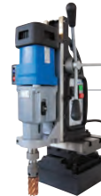
MAB 825 KTS p. 42 Capacity: \varnothing 3-1/8" cutter; \varnothing 1-1/4" twist drill; \varnothing 1-3/16" tapping Multi-axis positioning for boring, slotting, etc. Reversible, 4-gear motor
