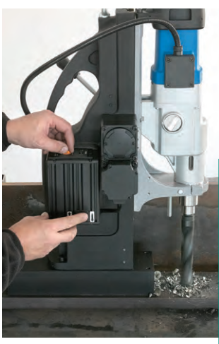
Automatic feed motor
