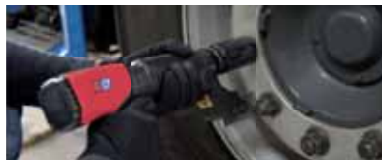
STEP 10 To ensure each nut has been torqued, a clockwise check may be performed. The BlueTork is pre-calibrated and is designed for precise torquing.
