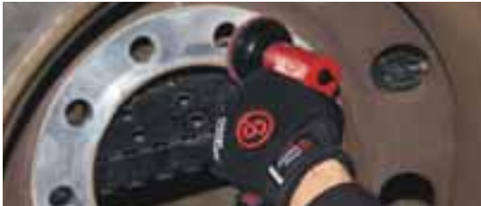
STEP 3 Thoroughly clean both sides of each wheel with the CP7202 sander and an appropriate abrasive. Inspect all surfaces for cracks and unusual wear.
