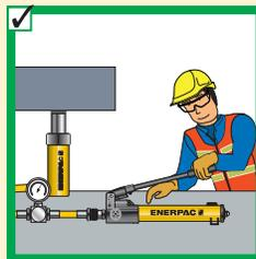
Don't use handle extenders. Hand pumps should be easy to operate when used correctly.
