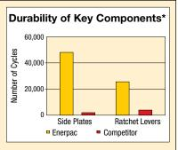
\*Average test results, whereby three Enerpac 1<sup>13</sup>/<sub>16</sub>" UltraSlim cassettes and three competitor 1<sup>13</sup>/<sub>16</sub>" cassettes were tested at 4000 ft-lbs for 50,000 cycles. The Enerpac side plates never broke for the full duration of the test.
