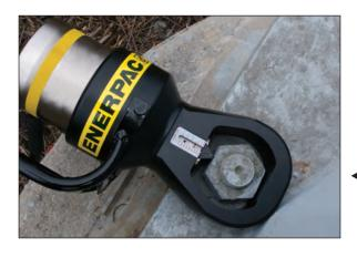
Heavily corroded and weathered nuts are quickly split and removed using an NS-Series Nut Splitter.
