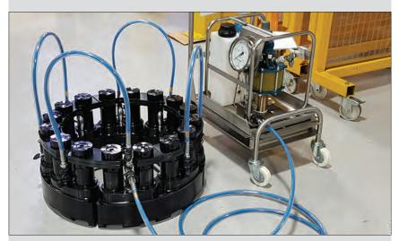
▲ Multi Stud Tensioning Set-Up.
