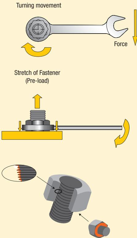
Friction points should always be lubricated when using the torque tightening method.
