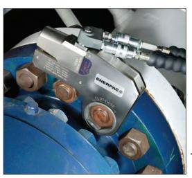
The ZE4 torque wrench pumps are perfectly matched for this W2000X wrench.
