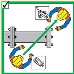
◀ The torque wrench (or tool) operator is always in charge.
