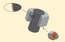
Friction points should always be lubricated when using the torque tightening method.
