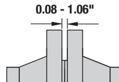
A mechanical tool for small diameter, low pressure flanges with a minimum access gap of 0.08 inch.
