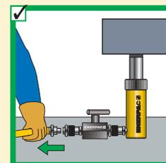
Detach cylinder only when fully retracted or use shut-off valves or safety valves to lock-in cylinder pressure.
