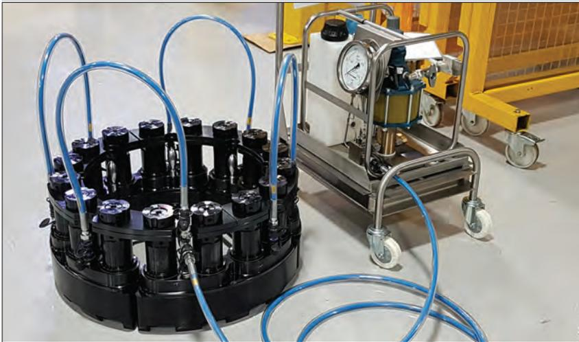
▲ *Multi Stud Tensioning Set-Up.*
