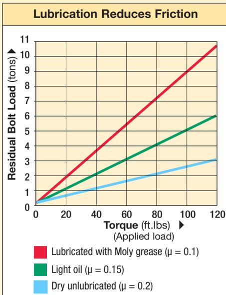
Example of how a lubricant can reduce the effect of friction and convert more torque to bolt preload.
