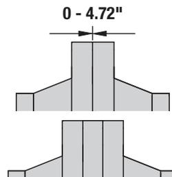
A unique flange spreader that is ideal for situations where there is no access gap or where there is a spacer, a wafer or butterfly valve positioned between the flanges.
