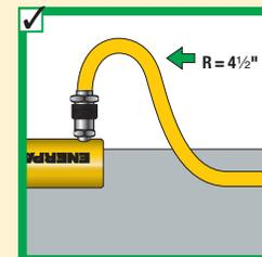
Don't kink hoses. Bending radius should be at least 4 1/2 inch. Don't drive over or drop heavy objects on hoses.
