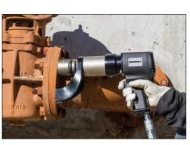
The PTW1000 makes quick work of this flange maintenance job.
