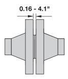
An innovative flange spreading wedge for use on small, medium or large flange joints with a minimum access gap of 0.16". The SWi range includes ATEX approved options.
