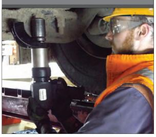
Safe and Quiet Axle Correction with a Pneumatic Torque Wrench.
