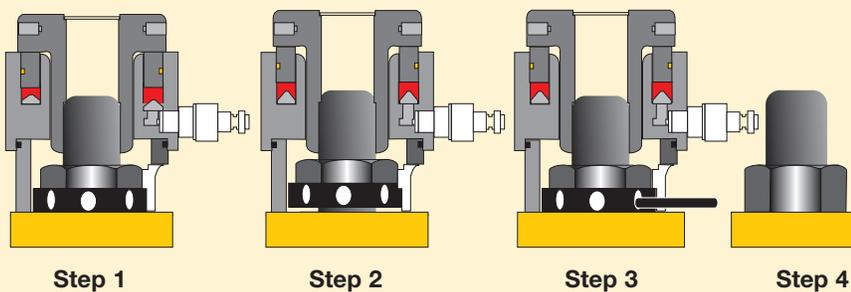
**Step 1:** The bolt Tensioner is fitted over the stud.
