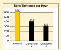
Internal laboratory testing based on standard torquing procedure on a pipe flange with 14, 17%" bolts.
