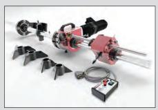
▲ Line boring machines for power generation and maintenance of construction vehicles.
