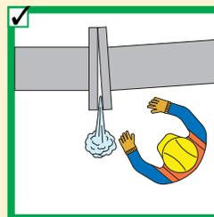
◀ Never stand in-line with the flange or pipe opening.
