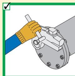
◀ Hold torque wrench (or tool) at handle only. Do not place any part of body between wrench and reaction point.
