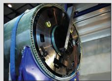
▲ Orbital milling machines for wind turbine manufacture.
