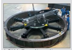
Orbital milling machines used in shipbuilding and power generation industries.
