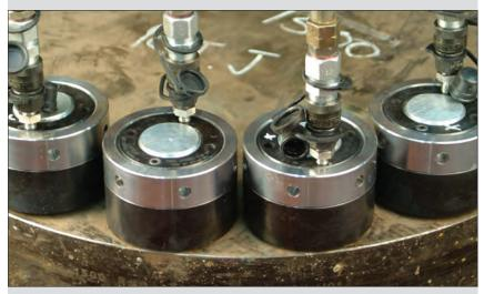
▲ Tensioning with hydraulic nuts.
