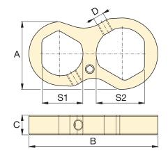
▼ Enerpac Back-Up Spanners to be used to stop back nut from turning during make up or break out.
