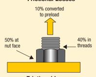
Frictional Losses (dry steel bolt)
