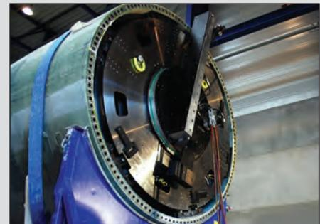
▲ Orbital milling machines for wind turbine manufacture.
