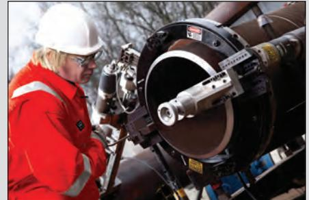
▲ Pipe cutters and weld preparation.
