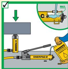
Fill pump only to recommended level. Fill only when connected cylinder is fully retracted.
