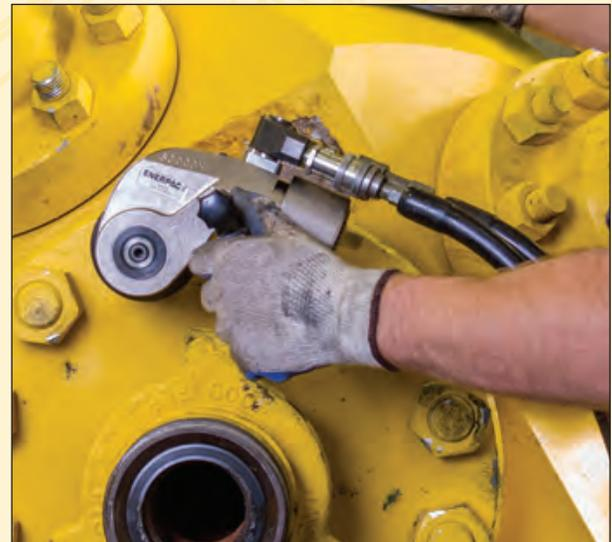
▼ RSL Drive Units with interchangeable RLP Hexagon Cassette and RSQ Square Drive Head
