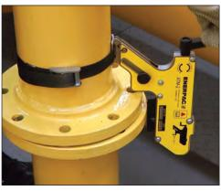
▼ The ATM-9 is shown here with optional pressure gauge and gauge adaptor.
