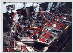
Hydraulic nuts on a diesel engine.
