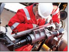
High torque portable drilling machines.
