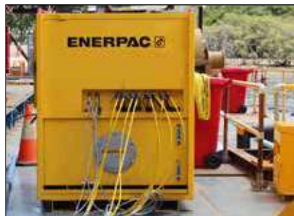
▼ SyncHoist Powerpack to operate the 4 lifting points.
