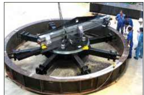
▼ Machining crane bearing face.
