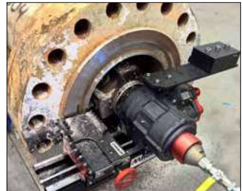
▼ MM860I machine to ensure flange joint integrity.
