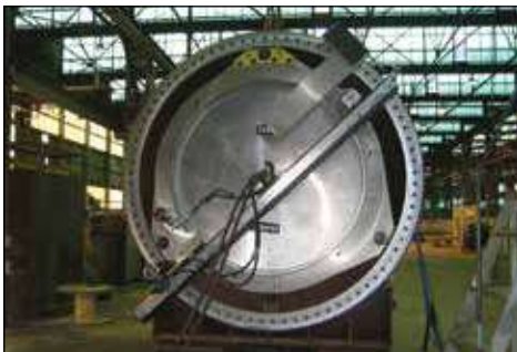
▼ Wind tower machining with WP4600.
