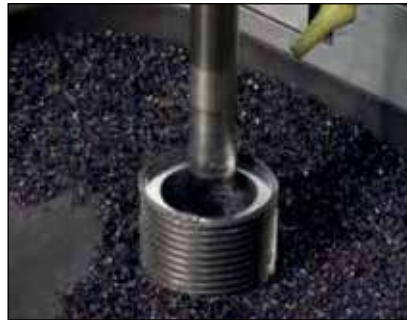
▲ Coring out the center of a bolt (minor diameter).
