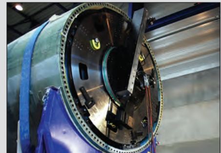
▲ Orbital milling machines for wind turbine manufacture.
