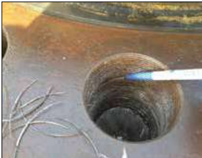
▲ A typical thread before refurbishment
