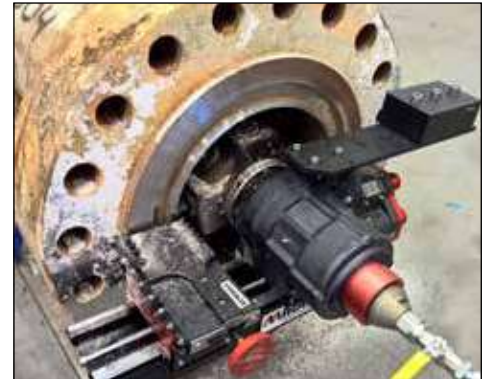
▼ MM860I machine to ensure flange joint integrity.
