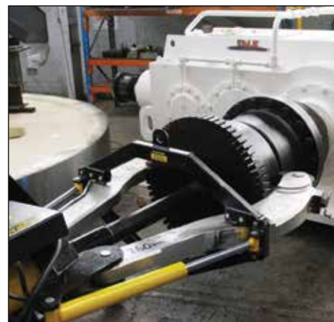
▲ The EPH1002 quickly and easily removes this drive coupler from its shaft.
