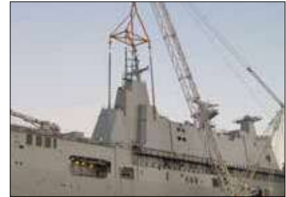
Synchronous hoisting and load positioning
