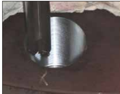
▲ New machined thread
