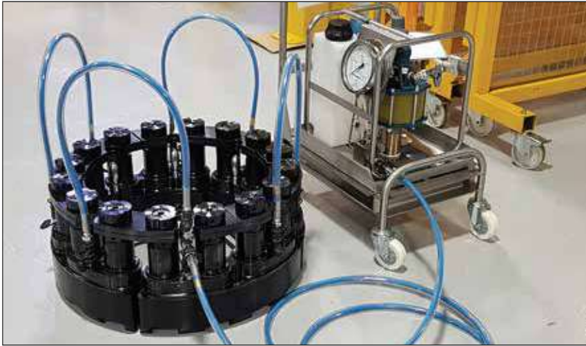
▲ Multi Stud Tensioning Set-Up.
