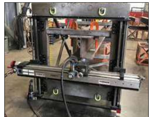
I-Beam end face milling with a GMRF1000. ▶
