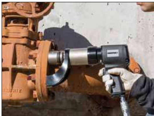
◀ The PTW1000 makes quick work of this flange maintenance job.
