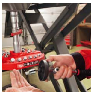
3 Drain plug dripping above the oil collector.
