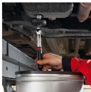
2 Drain plug removal completed in driver position, oil drops are stopped by the protection cup.
