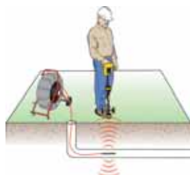
Find sondes (remote transmitters).
