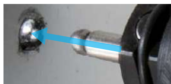
Insert rivet into the hole.
