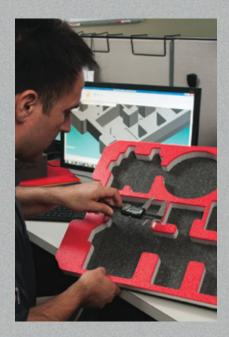
Our Pelican Case Centers have the most advanced foam cutting tools, and our engineers have the latest software applications so they are able to create a design that is precise and determines the most cost effective method of manufacture.
