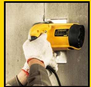
5 Slotting On Wall; Cutting Ceramic Tile Tile Cutter STSP125
